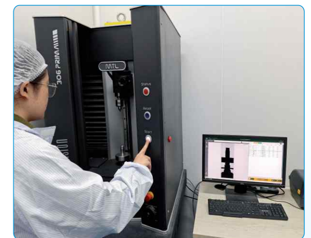
Axial Scanner Stretching process control to ensure dimensional and shape control during the stretching process
